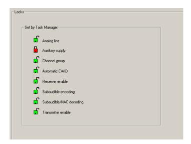
Analog line When the analog line is locked, the analog line cannot be used.
